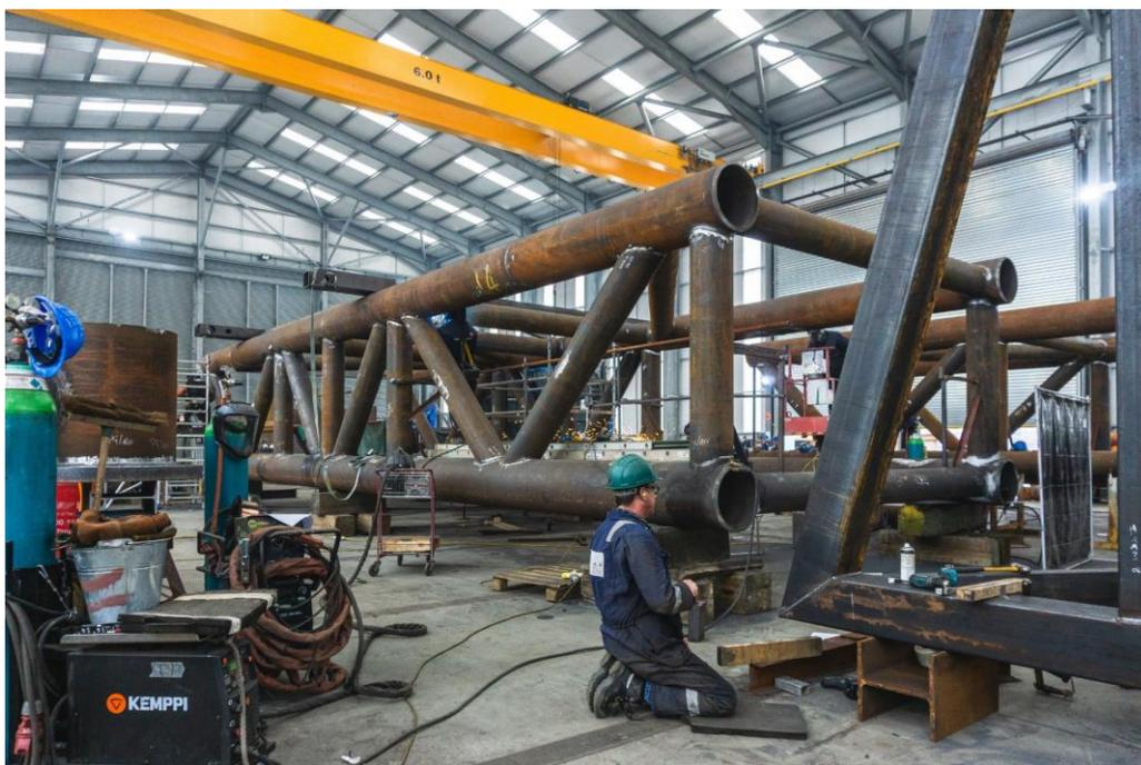
**Image Caption:** mWave fabrication nearing completion at Mainstay Marine's workshop in Pembroke Dock.
