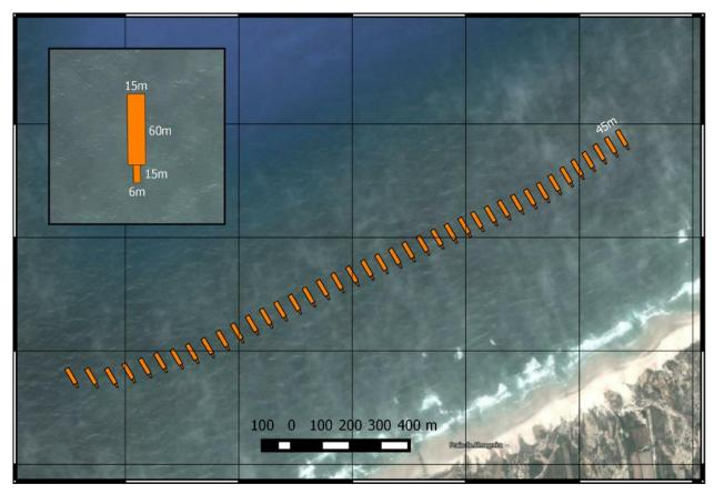
Figure 1 – Bombora's 60MW mWave Farm Configuration
