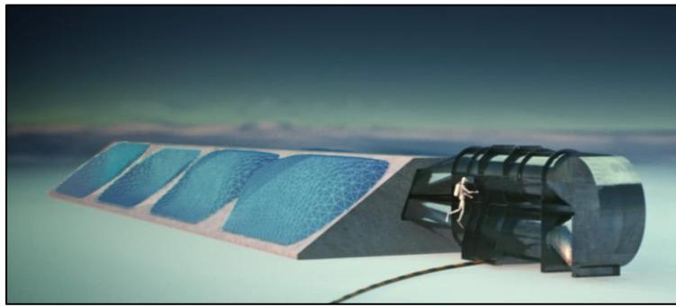
**Resting on the seafloor at a depth of 10 metres, the rolling membrane of the mWave™, converts wave energy into pressurised air which passes through the turbine to produce electricity**
